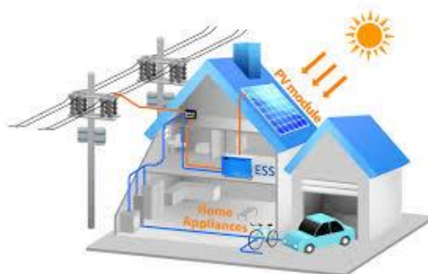
Figure 29 - The Prosumer concept. The Power transmission goes from one-way to two-way lines
