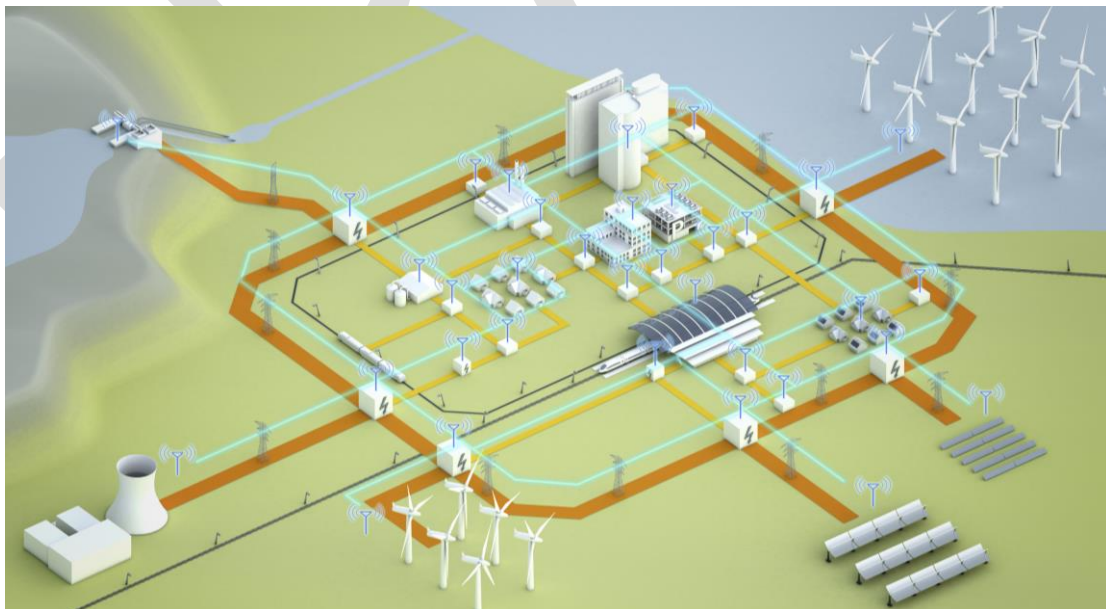
Figure 28 - Smart Energy landscape – from centralised to distributed (PV, wind, biogas, ...) generation and conversion, consisting of High/Medium Voltage grid (orange), Low Voltage grid
