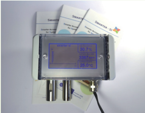
Indoor air control measuring system (left) with an integrated CO2 sensitive colour changing foil (right)
