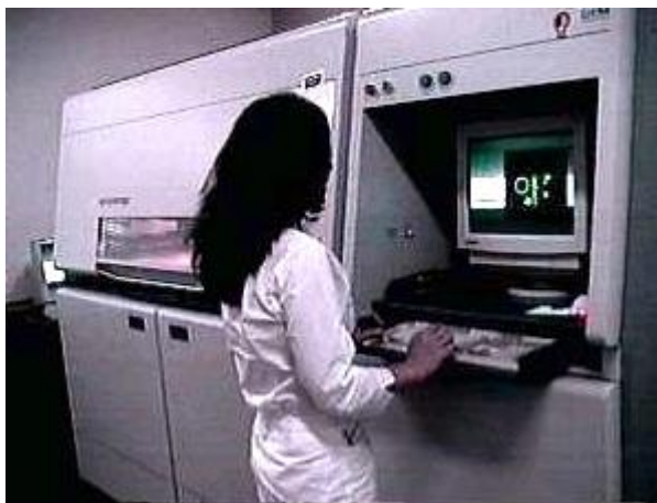
A rapid prototyping machine using selective laser sintering Photo: Renato M.E. Sabbatini
