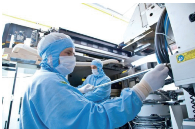
Figure 1. Integration of projection optics in ASML TWINSKAN Wafer Scanner. Source: ASML.
