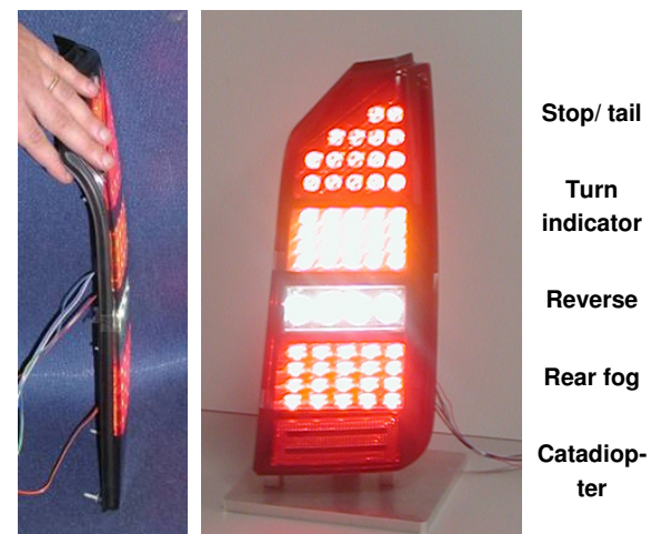
Figure 3: Lighting system based on solid state emitting sources, novel nanoscaled high efficiency phosphors and planar micro optics integrated directly on the external polymeric cover.
