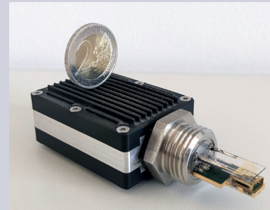
MEMS based fluid sensor (demonstrator) © Fraunhofer ENAS
