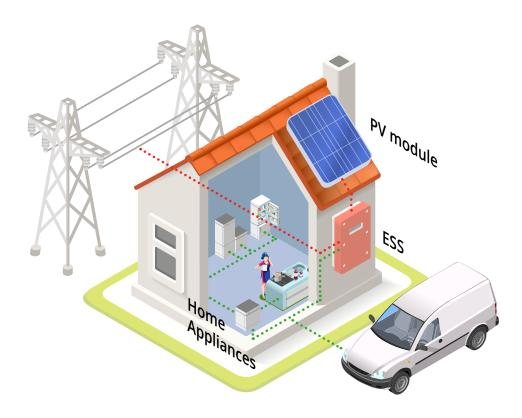
The Prosumer concept. The Power transmission goes from one-way to two-way lines.
